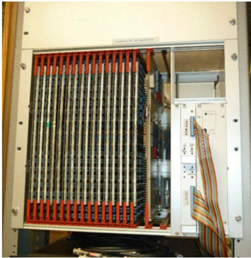
Fig. 5. The complex apparatus which formed the 500 MFlops digital dedisperser (Andrea Maccaferri).
